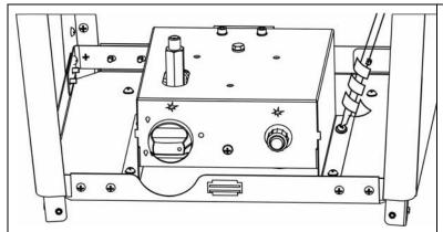
**STEP 2:** Lay down tank housing, fix the Burner Assembly (9) to Pate Cover (8) by 4pcs M5 Screws and Washers (BB).
