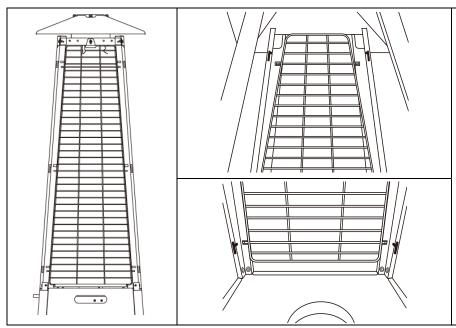
**STEP 8:** Insert 6 projecting ends of each Mesh Guard (4) into the seat slots of Support Bar–Upper (3) as shown in picture. Fix all Mesh Guards (4) except the front side.
