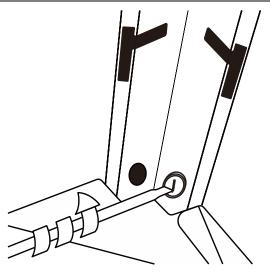
**STEP 7:** Place the whole upper parts to top of tank housing assembly. Make sure match the top ends of tank housing assembly with the bottom slot of Support Bar – Upper (3). Match the threaded holes and fix each connection with 2pcs M5 Screws and Washers (BB)
