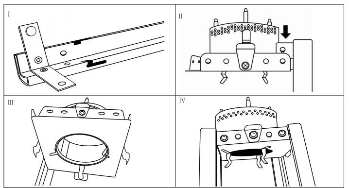
**STEP 5:** Attach Flame Screen (2) to the top of Support Bar-Upper (3) and fix the connection with 2pcs M5 screws and washers (BB), (See Figure I, II).
