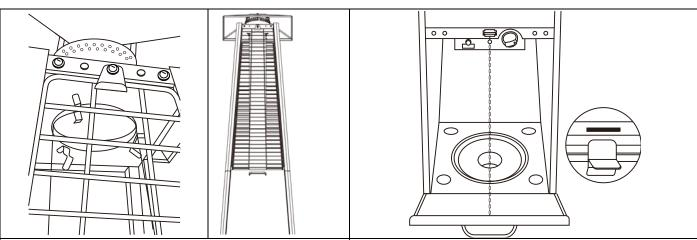
**STEP 10:** Assemble Mesh Guard (4) in the front. Loose 4pcs screws to keep 4pcs Guard Fastening Plates down and firmly in place.
